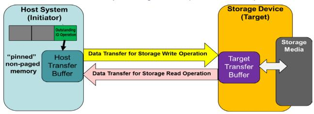
IO Queue Memory = IO Queue Depth \* size of (IOP Descriptor + Transfer Buffer)
