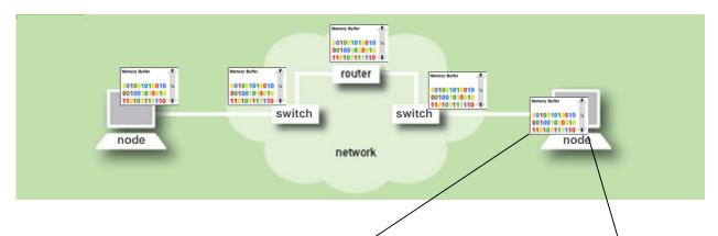
This can lead to a Buffer Overflow resulting in Data Packet Drops forcing error recovery delays.
